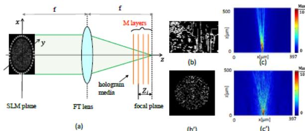
Figure 1: (a) Simulation model of hologram recording process, (b) image with conventional preprocessing, (b') random arrangement of (b), (c) and (c') cross sections of intensity distribution in holographic media where (b) and (b'), respectively, were the inputs. SLM: spatial light modulator.
