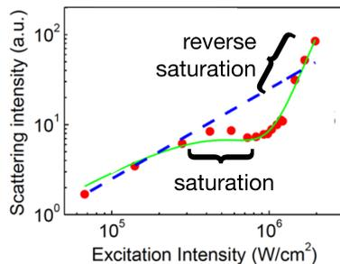
**Fig. 1:** The nonlinear scattering response from a single gold nanoparticle with 80 nm diameter [3]. Green line shows the polynomial fitting.
