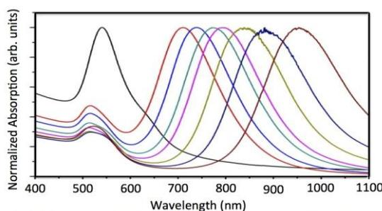
Fig. 1 shows Gold nanostructures peak scattering (extinction) can be tuned across the visible and near IR spectra.
