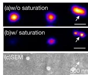
**Fig. 2:** The comparison of scattering images of gold nanoparticles [3]. The diameter of particles is 100 nm. (a) Conventional confocal image without saturation. (b) The image with saturation method. (c) Scanning electron microscope (SEM) image.
