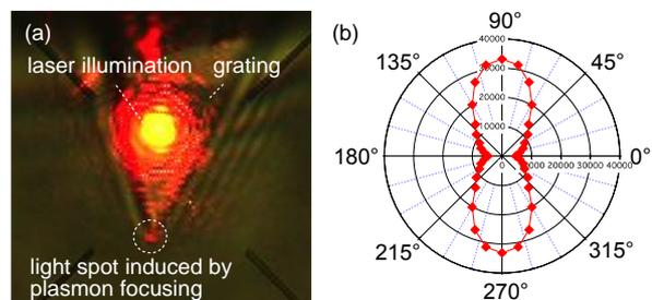
**Fig. 2:** (a) Optical image of a light spot induced at the apex through plasmon focusing. (b) Intensity of near-field light with respect to incident polarization.
