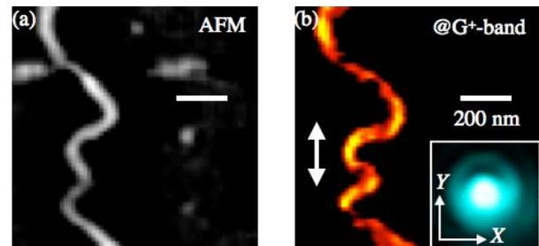
**Fig. 2:** (a) AFM and (b) TERS images of SWNTs. The white arrow in (a) means the in-plane component of the dipole oscillation induced in the tip used in the measurement. Inset shows the defocused image of the dipole indicating the oscillation direction.
