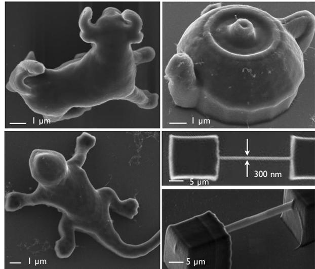
**Fig. 1:** SEM images of 3D micro structural SWCNT/polymer composites
