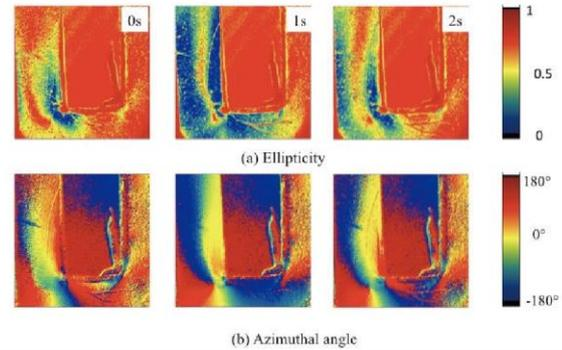
**Fig. 2:** Dynamic measurement of ellipticity and azimuthal angle of polarization of U-shape film.
