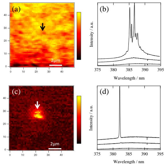
**Fig. 2:** Emission distribution and emission spectra at the defects within (a,b) non-treated and (c,d) laser-treated ZnO NP films. In (b) and (d), The excitation intensities were 0.5, 1.0, and 2.0 times of each threshold, and appropriate offsets were added for the sake of clarity. Arrows represent the positions of a point defect.
