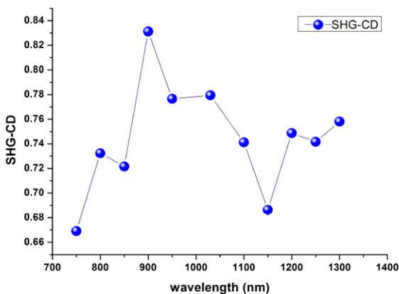
**Fig. 1.** SHG-CD value varies with the excitation wavelength from 750 to 1300nm.
