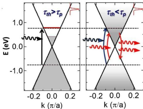
**Fig. 1:** Dispersion of electron-doped graphene monolayer illustrating state filling (left) and band filling (right) that leads to stimulated emission from a broadband, inverted population (red arrow).
