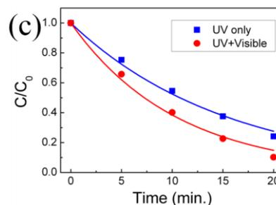
**Fig. 2:** The relative concentration at different time of reaction with and without visible light source. C is the concentration of MO molecules at time t, and C<sub>0</sub> is the original concentration.
