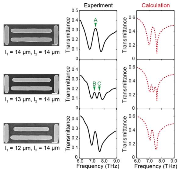
**Fig. 2:** Transmittance spectra in dependence on the wire length  $l_1$ . Left column shows SEM images of the corresponding structures. Black and red curves represent the experimental and calculated transmittance spectra, respectively.
