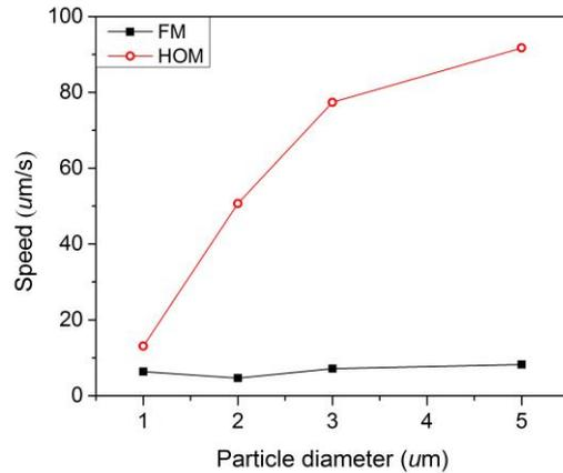
**Fig.2.** Speed dependence on particle size under both HOM (red circles) and FM (black squares) propagation. In both cases the waist power was 25 mW.
