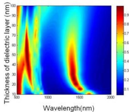
**Fig. 2:** Absorption spectra for VSRR-based super absorber as a function of thickness of dielectric layer. A pronounced resonance peak associated magnetic dipolar response around 1.5  $\mu\text{m}$  is recorded which can be employed for super absorber application in optical region.
