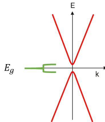
**Fig. 2:** Band gap appearance when graphene is shone with circularly polarized laser field. The band gap is proportional to the intensity of the field and inversely proportional to the frequency.
