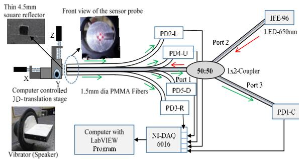
**Fig. 1.** Schematic experimental setup of the seismic vibration sensor.
