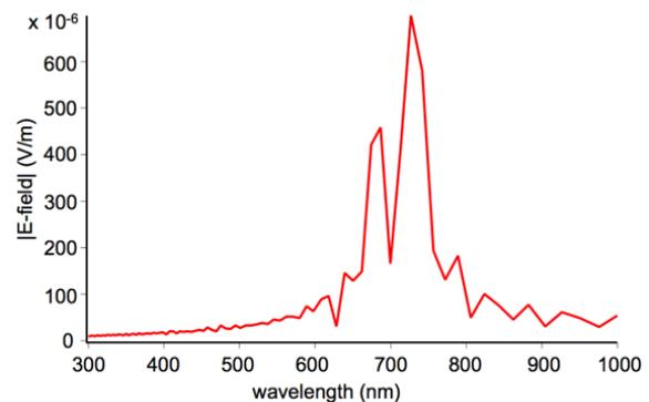
**Fig. 2.** FDTD calculation of E-field at the output side of 11 aligned Au nanorods chain in air. The strongest peak appeared at 727 nm.
