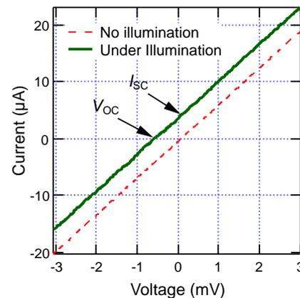
**Fig. 2:** I-V characteristics of the CNT fiber photodetector with (green line) and without (red dashed line) illumination at 660 nm.
