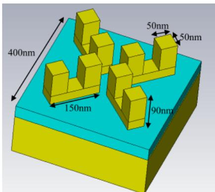
**Fig. 1:** Schematic diagram for VSRR-based super absorber device. A unit cell composed of four VSRR structures with identical dimensions.
