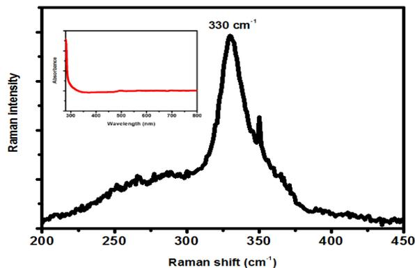
Fig.1: Raman spectrum of CZTS nanocrystals. Insert shows the absorbance of CZTS nanocrystals.
