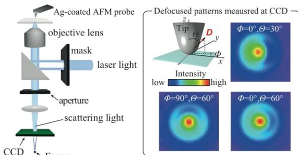
**Fig. 1:** Overview of defocused imaging to investigate the dipole induced at the apex of a TERS tip.
