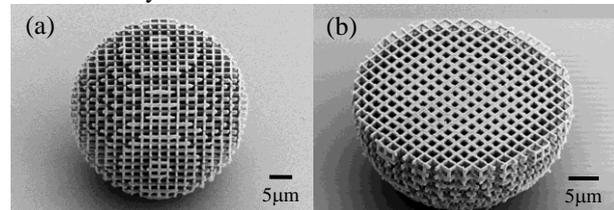
**Fig. 2:** SEM image of the fabricated Luneburg lens. The radius of 3D Luneburg lens is 20  $\mu\text{m}$ . The distance from the top of the lens to substrate is 40  $\mu\text{m}$ . (a) Overall drawing, (b) Internal sectional drawing.
