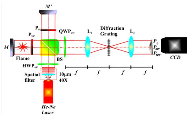
**Figure 1** Setup of the instantaneous polarized phase-shifting interferometer
