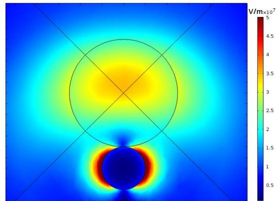
**Fig. 2:** LSPR of a 200 nm gold particle (lower circle) excited with light of wavelength 808 nm near a 500 nm MNF (upper circle).
