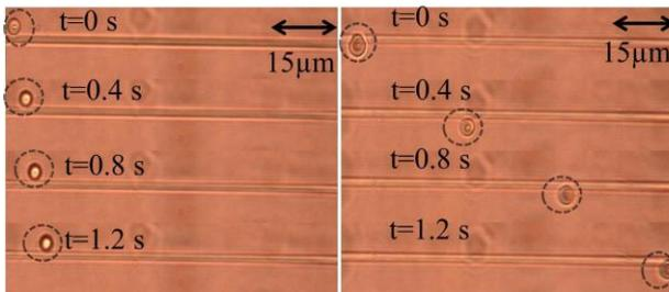
**Fig.1.** Micrograph for the speed of a 3  $\mu\text{m}$  diameter polystyrene particle (marked with dotted circle) under FM (left) and HOM (right) propagation. In both cases the waist power was 25 mW.
