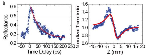
**Fig. 2:** (a) Measured reflectance changes of a 1550 nm probe laser as a function of delay time between pump and probe pulses (b) Measured closed-aperture Z-scan curve of a 180-nm-thick ITO film.
