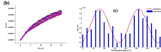
**Fig. 2:** (a) Mechanism of measurements. (b) the I-V curves of MoS<sub>2</sub> FET with different incident polarization angle from 0° to 180°. (c) The Drain-Source current ( $V_{ds}=5V$ ,  $V_g=-30V$ ) was manipulated by a polarized incident laser.
