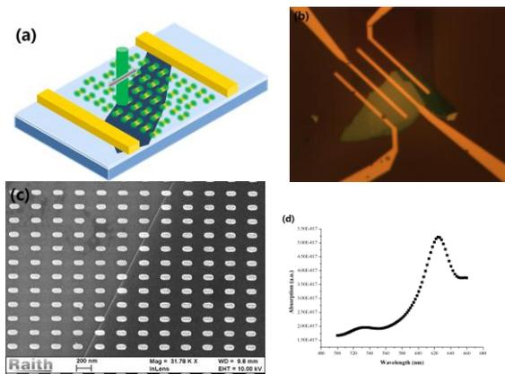
**Fig. 1:** (a) Configuration of nanobar coated MoS<sub>2</sub> FET. (b) Optical image of multilayer MoS<sub>2</sub> FET. (c) SEM image of nanobar array (single nanobar size: 50nm:50m:100nm). (d) Simulated absorption spectrum of Au nanobars by Comsol Multiphysics software.
