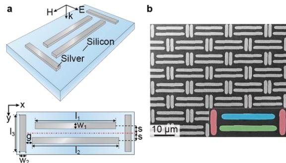
**Fig. 1:** Structural geometry of PIT metamaterials (a) Schematic diagram of the metamaterial. (b) Normal view of the structure. Inset: Enlarged view. The dipole antennas are indicated in red and quadrupole antennas are indicated in blue and green, respectively.
