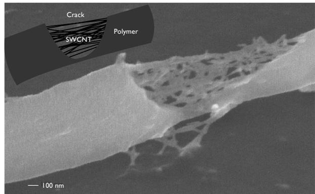
**Fig.2:** SEM image at a crack on a nanowire produced by laser ablation. SWCNTs are bridged between the crack.
