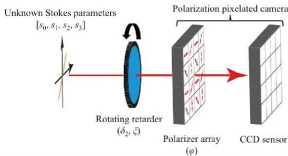
**Fig. 1:** Optical setup of Stokes polarimeter using the rotating retarder and polarization pixelated camera.
