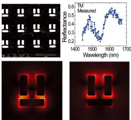
**Fig. 1:** (a). SEM image of the metamaterial. (b) Measured linear reflectance spectrum of the metamaterial for TM polarization incidence case. Calculated electric-field distribution of the meta-molecule for the TM-polarized incident light with a wavelength of 1460 nm (c), and 1550 nm(d).
