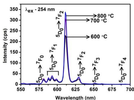
Figure 1 Emission spectra of  $\text{Gd}_2\text{O}_3:\text{Eu}^{3+}$
