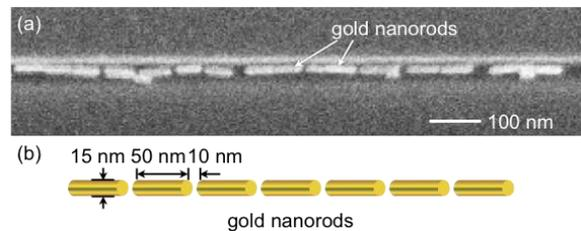
**Fig. 1.** (a) SEM image of self-assembled Au nanorods in a thin trench (b) Aligned Au nanorods of 50 nm heights, 15 nm diameters and 10 nm gaps.
