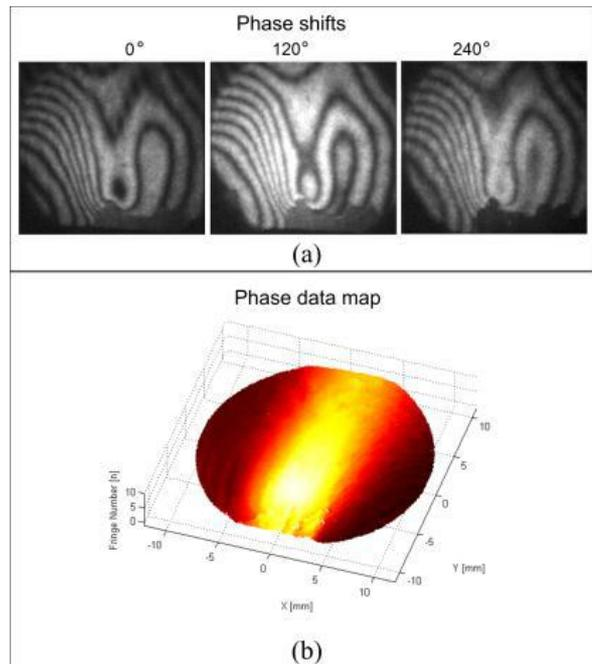
**Figure 2** a) Three phase shifted interferograms obtained in a single capture and b) Unwrapped Phase map.
