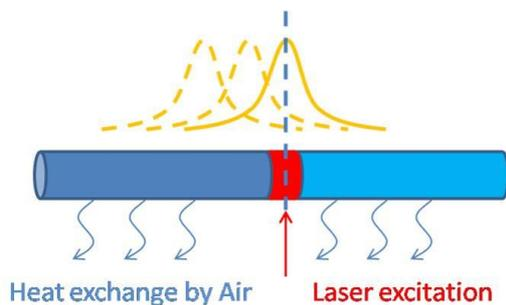
**Fig. 1:** Photodetection with a CNT fiber. The fiber is illuminated at the junction (red), and heat is produced, generating a voltage via the Seebeck coefficient gradient. Solid and dashed brown lines are temperature profiles due to illumination at different positions.
