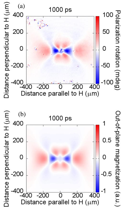
**Fig. 1:** (a) Measured map of the Faraday rotation of probe pulses.
