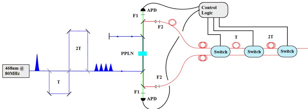
**Figure 1** – Schematic of the hybrid multiplexed source. PPLN; periodically poled lithium niobate crystal, F1; narrowband filter centred on 671nm, F2; narrowband filter centred on 1547.5, T; 3.125ns delay,  $\Delta T$ ; fibre delay to match arm 1 and 2, APD; avalanche photodiode detector.
