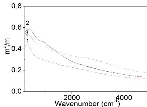
**Fig. 2:** Frequency dependences of effective mass  $m^*/m$  of ZnO films for different Er-content (1- 0.64% Er, 2- 0.9% Er, 3-1.2% Er).
