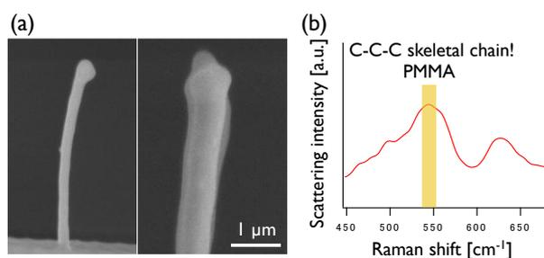
**Fig. 1:** (a) A set of polymer wires with different nanosized wire radii. (b) A Raman spectrum obtained from a polymer wire.
