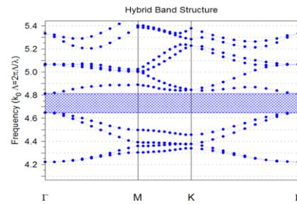
Fig. 1: Band structure of proposed PBGF for  $n_b > n_r$ .
