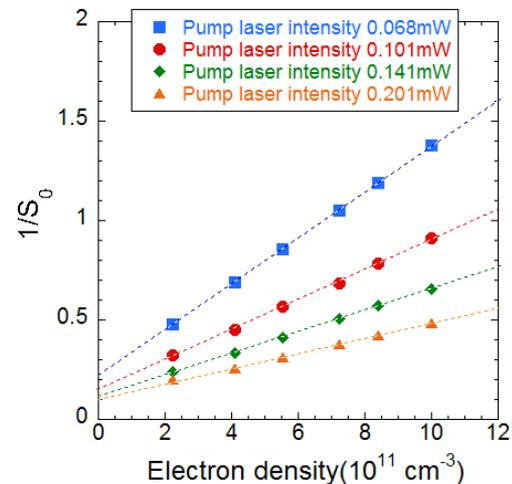
**Fig. 1:** Relationship between the reciprocal of the saturation parameter and the electron density. (Argon gas pressure is 100mTorr)
