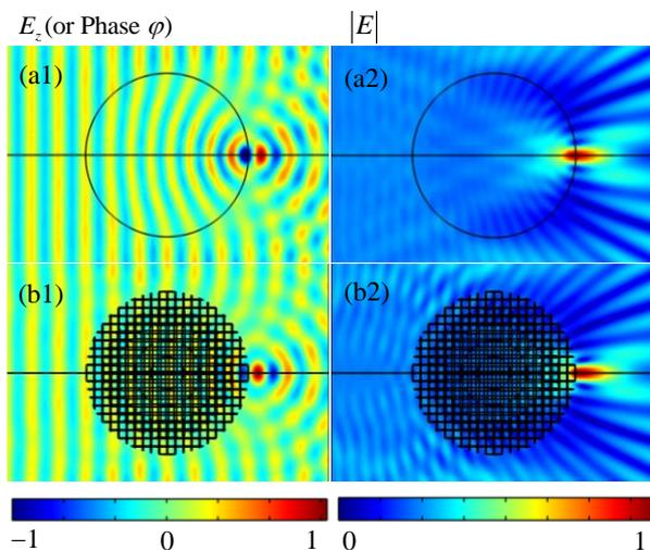
**Fig. 1:** FEM simulation results of electric field distribution for (a) the original ideal lens and (b) the GRIN PCs based on Luneburg lens, The incident
