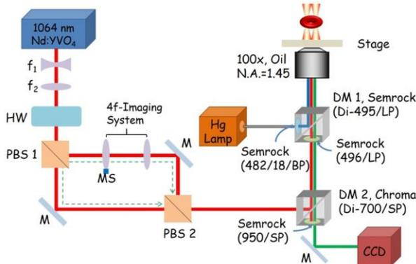
**Fig.1:** A schematic diagram illustrating the integration of a dual-trap optical tweezers with a fluorescence microscope.
