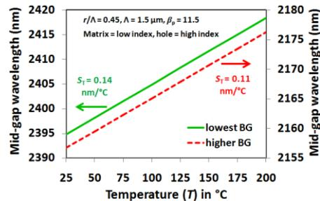
Fig. 3:  $T$  dependent of mid-gap  $\lambda$ . Green solid is for lowest BG and red dashed is for higher BG.
