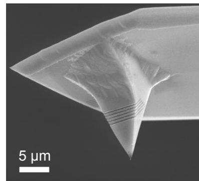
**Fig. 1:** SEM image of a silver-coated tip with a grating structure.
