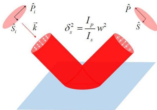
**Fig.1:** The relationship between SHEL and cross polarizations. An  $S$  polarized Gaussian beam impinges upon an interface and is reflected. The polarization of reflected beam is spatially variant in the wave front. The total intensities of reflected beam that along  $P$  polarization and  $S$  polarization are related to the SHEL
