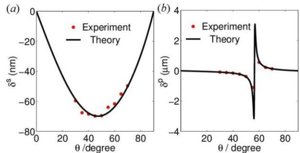
**Fig.2:** SHEL displacements of left-handed component, as a function of the incident angle  $\theta$ , in the case of (a)  $S$  polarization and (b)  $P$  polarization. The dots are experimental results, and solid curves are theoretical prediction.
