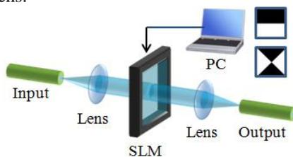
Fig. 1: Conceptual design of the phase modulation method.
