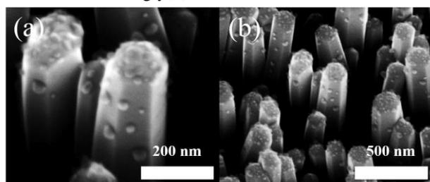
**Fig. 1:** (a, b) The SEM images of silver-sputtered ZnO nanorods. The sizes of the silver nanoparticles range from 10 to 45 nm.
