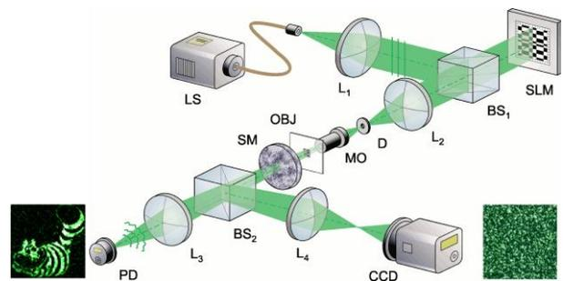
**Fig. 1:** Disorder-assisted compressive microscopy. Schematic diagram of the optical setup. The object is the *Cheshire Cat* from *Alice's Adventures in Wonderland*.
