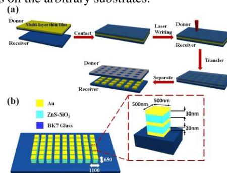
**Fig. 1:** (a) Schematic illustration of fs-LIFT process. (b) The feature size of a multilayered plasmonic cavity in nanometer scale. The period along x-direction  $P_x$  and y-direction  $P_y$  are 1100 nm and 650 nm.
